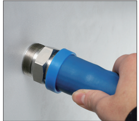
3. Hold end connection against flat surface, Grip hose and push with a steady force until hose seats into blue finishing.
