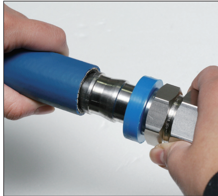
2. Cover first barb of end connection with hose. (Lubrication fitting stem with light oil may ease assembly)
