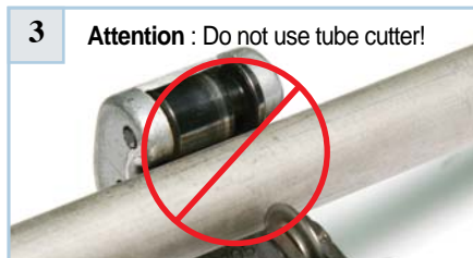
3 Attention : Do not use tube cutter! a) tube cut with tube cutter : heavy burr / bevel cut
