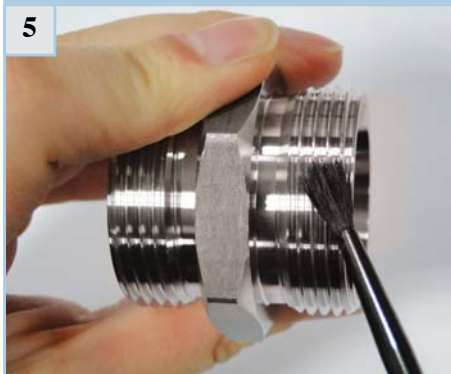
Lubricate thread and cone of fitting body, also compression ring and thread of nut.
