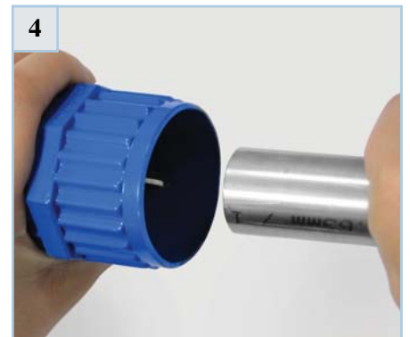
4 Lightly de - burr inside and outside edge. Bevel up to 0.3mm × 45° (0.012" × 45°) permissible.
