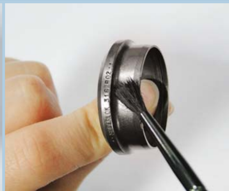
Lubricate thread and cone of fitting body, also compression ring and thread of nut.
